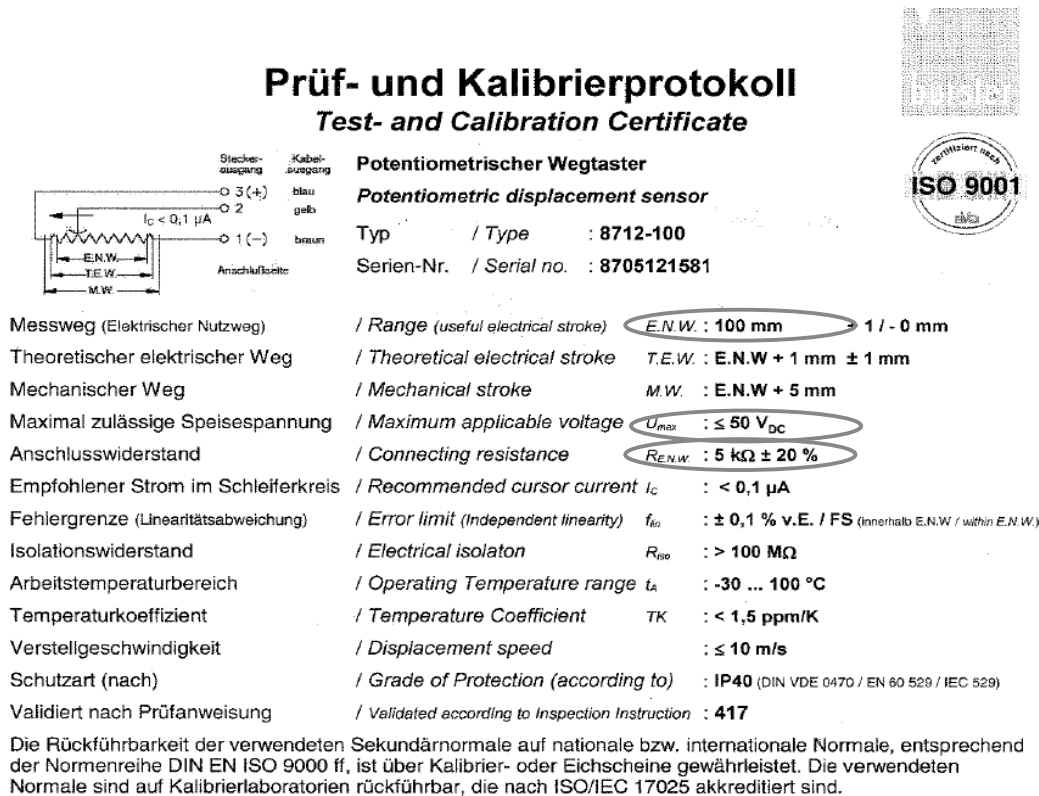
Figure 22: Test and calibration certificate for a potentiometric position sensor
